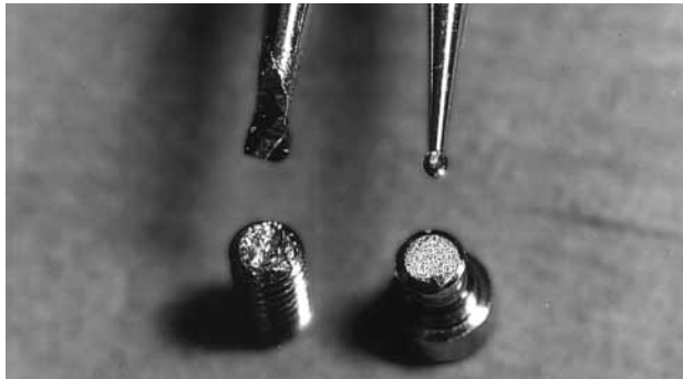
Fig. 3. Retrieved fractured implant screw with groove.
